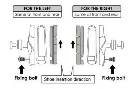
Tighten the fixing bolt. Tightening torque: 1-1.5 Nm.
